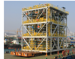
Figure 5 - CO 2 unit using the UOP spiral wound membrane
